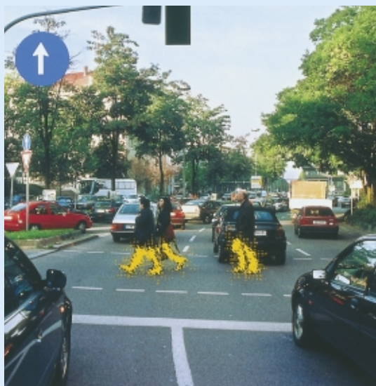
Pedestrians are recognized from their typical leg movements. The system uses picture sequences for identification.
